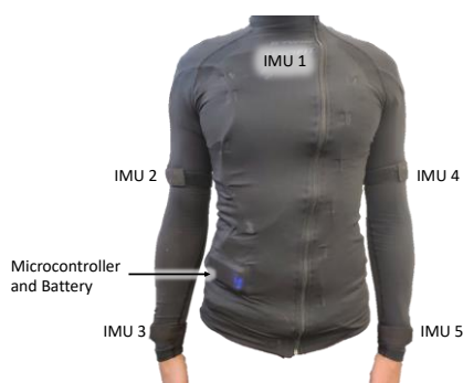
Figure 1. First prototype of the ArmTracker system with 5 IMU sensors, a microcontroller and a battery.
