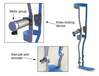
Fig. 1. CAD design of the first prototype of active KAFO.
