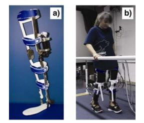
Fig. 2. (a) Prototype with femur-aligned motor. (b) Experimental test of a SCI subject wearing the active KAFO.
