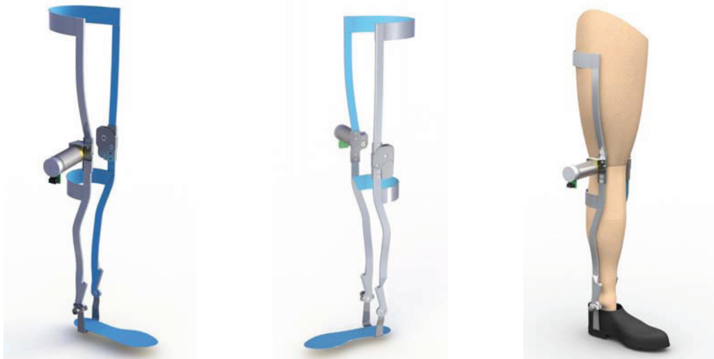
Fig. 9. Global mechanical design of the orthosis.
