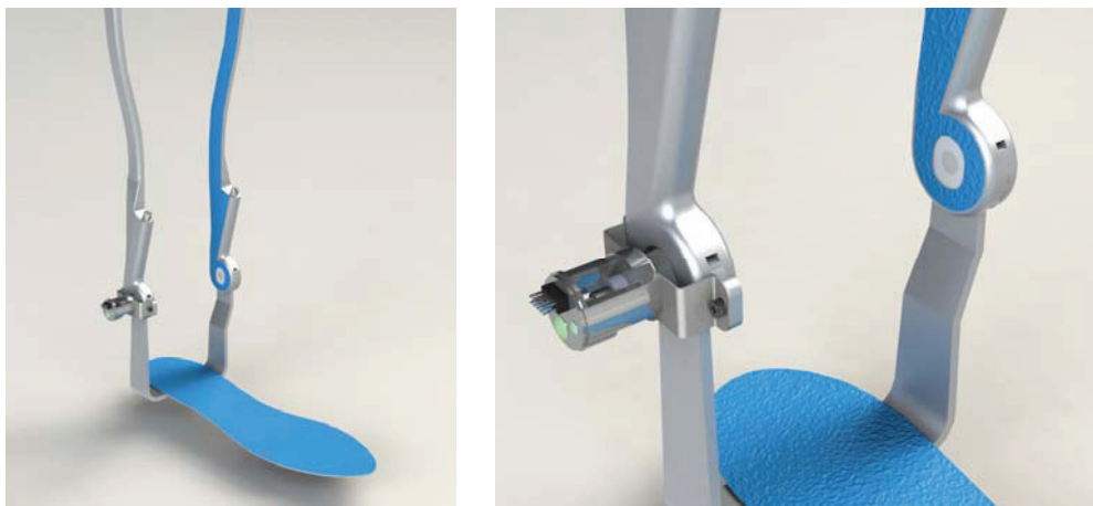
Fig. 7. Ankle unit of the A-SCKAFO and detail of the encoder placement.
