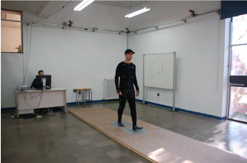
Figure 3-4. Normal male subject performing a walking in the UPC Gait Lab
